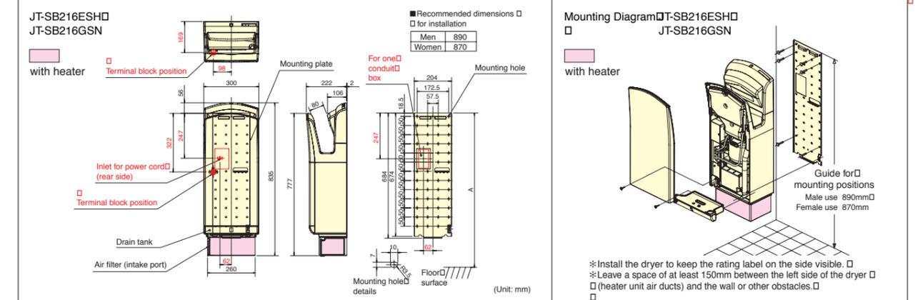
\*Because there is no power cord, pull the ø1.0~ø2.5 cable out of the wall by 450mm. \*Confirm points of caution about installation space with the dealer.
